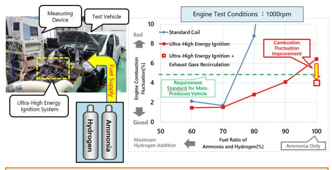
Establishment of stable combustion at 100% ammonia by making full use of ultra-high-energy ignition system and exhaust gas recirculation system.
